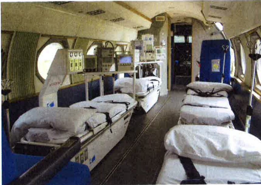
Phoenix Air Gulfstream III outfitted to handle up to five patients simultaneously.
